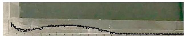
FIG. 1 (color online). A schematic of the system and an image of a simple experiment showing a propagating peeling front in a plastic shim on a layer of glycerine. Dark solid lines indicate experimental data; dashed lines are the result of solving (7) and (8) numerically. These plots show a snapshot in time as the plastic peels off the underlying substrate. Experimental parameters are \rho_f = 1.2 \text{ g/cm}^3 , \mu = 10 \text{ g/cm s} , Q = 3.3 \text{ cm}^2/\text{s} , E \approx 8.3 \times 10^{10} \text{ dynes/cm}^2 , b \approx 0.1 \text{ mm} , \Delta\rho = 5 \text{ g/cm}^3 . This corresponds to H_g = 2.0 \text{ cm} , L_g = 12.0 \text{ cm} , and \mathcal{G} = 283.2 .
