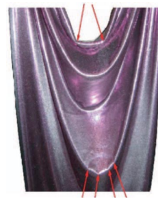
FIG. 1 (color online). Condensation of curvature in a heavy drape. The smooth catenarylike folds with a single direction of localized curvature coexist with regions of curvature condensation, indicated by arrows, where curvature is strongly focused.
