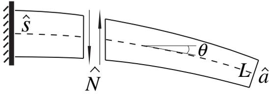
Fig. 1: A cantilevered branch showing the geometry and notation:  $\hat{s}$  is the arc length,  $\hat{s} \in (0, L)$ ,  $\hat{N}$  is the vertical shear force,  $\hat{a}$  is the cross-sectional area profile,  $\theta$  is the angle of the center line tangent with the horizontal direction.
