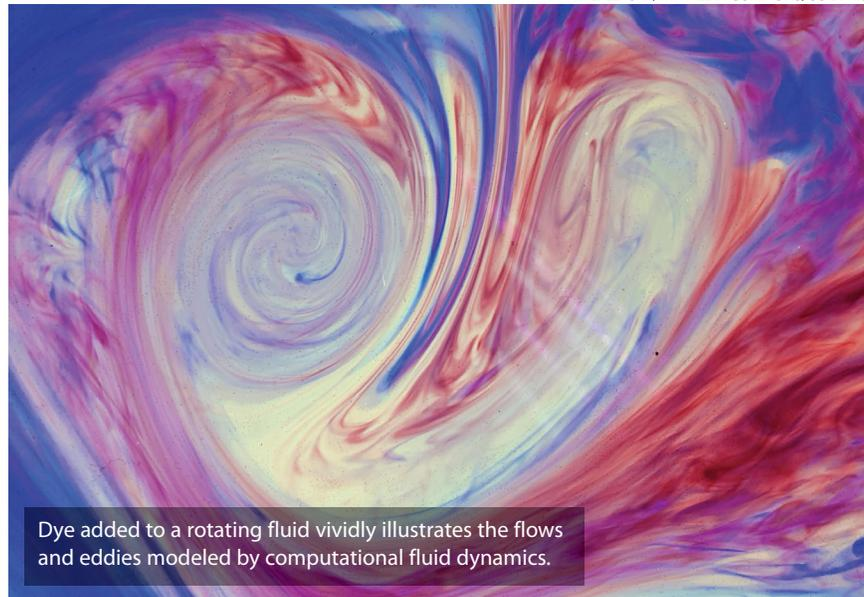
Dye added to a rotating fluid vividly illustrates the flows and eddies modeled by computational fluid dynamics.
